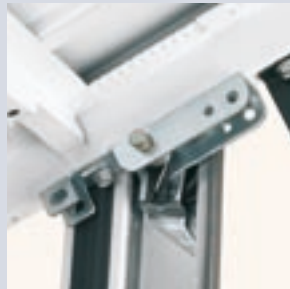
Anti-drop device to prevent the door from crashing down in the event of a spring or cable failure.
