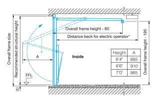
\* Distance back for ProMatic/SupraMatic electric operator: 3200 mm up to door height 2500 mm 3450 mm up to door height 2750 mm
