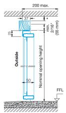
\* 40 mm headroom required for electric operator
