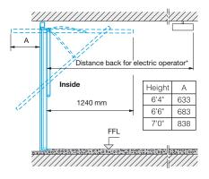
For doors with operator 40 mm headroom above top crossframe required. (Overall frame size + 40 mm)
