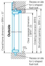
\* With an opening angle of less than 180°, the clear passage width is reduced.
