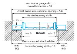
Behind opening installation with the Hörmann steel frame allows for a wider range of structural openings to be spanned, this can be particularly helpful with non-standard openings which would normally require special sized doors. The diagrams show the minimum tolerances that should be adhered to.
