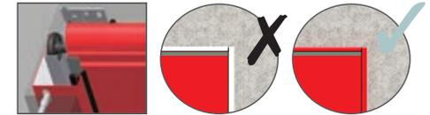
I'm fitting between the reveal, how do I cover the fixing holes?
