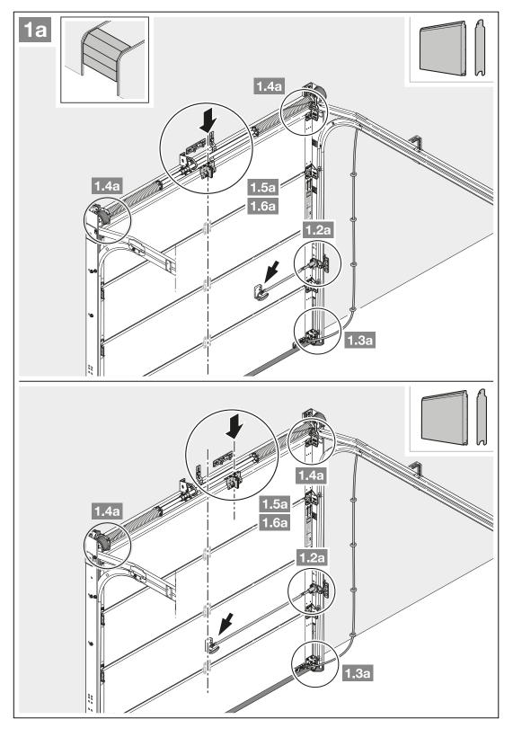
With an off-centre reinforcement profile, fit the link bracket on the nearest reinforcement profile to the left or right.
