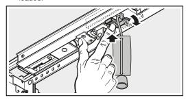
Push the green button on the slide carriage. The slide carriage is re-engaged for automatic operation.
