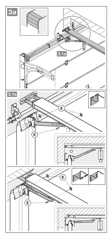
Depending on the **door type**, take the installation direction of the link bracket into account.
