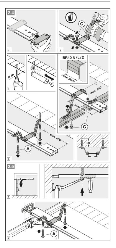
Depending on the **door hardware**, take the installation direction of the link bracket into account.
