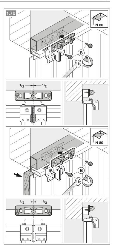
With N80 doors with timber infill, use the bottom holes on the lintel joint for fitting.
