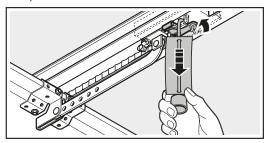
Pull on the cord of the mechanical release. The slide carriage is disengaged for manual operation.
