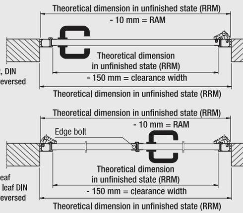
Installation behind the soffit, only inward opening
