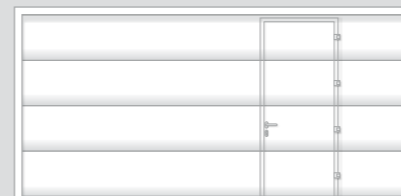
Asymmetrical arrangement for garage door widths above 3,500 mm – either left or right
