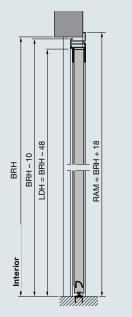
Side door with aluminium corner frame, profile type 2 External fitting
