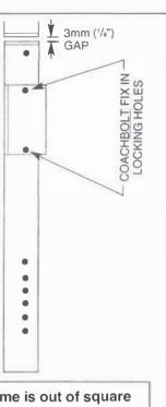
IMPORTANT. For proper operation the frame must be square. If the frame is out of square the bottom weather strip MUST be square to the door otherwise the door will not operate correctly.
