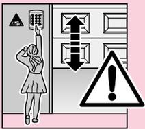
**Permanently installed controls (such as buttons or similar devices) should be installed within sight of the door but well away from any moving parts and at a height of at least 1.5 metres. It is vital that they are installed out of the reach of children!**
