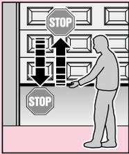
All persons using the door system must be shown how to operate the garage door opener properly and safely. Demonstrate and test the mechanical release as well as the safety return. **To do this, halt the closing door by grasping it with both hands. The door system should gently cut-out and initiate the safety return. The same should happen during the opening cycle, i.e. the door system gently cuts out and the door comes to a halt.**
