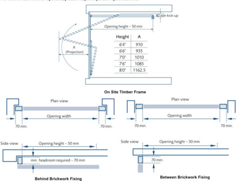
The garage door is supplied factory fitted to a steel box section frame and is secured to the brickwork using just 7 fixings.
