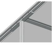
Image shows gutter channel fitted.
