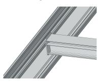
Starting with the End Glazing Bar, push this bar into the wall plate so that it is pushed back as far as possible and ensure the outside profile lines up with the edge of the wall plate. Rest the other end of the glazing bar on the radius inner section of the gutter section.
