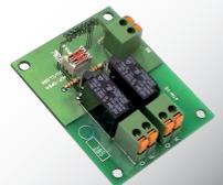
Modul „GT“: provides either separated impulses for opening and closing operations OR a partial opening feature which is handy for side-running sectional doors.
