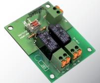
Modul „AZ“: provides advanced features for automatic closing. Fast-closing after passing the photo-cell or fixed closing times from 10 to 240 seconds adjustable.
