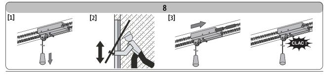
When disengaging the motor drive mechanism, use caution for a badly balanced door may cause sudden door movement that may be dangerous.
